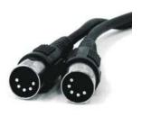
The **MIDI** standard grew out of the Audio Engineering Society in the early 1980s and was formally ratified as an industry standard in 1983. The interface allows for communication between digital instruments, computers, and other electronic devices, in order to produce sound. The MIDI interfaces themselves do not carry sound or produce music, but, rather, they carry sets of instructions for one device or another to produce the sound or music (including specific commands
