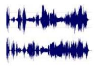
Compare this to an **audio** recording. A recording of sound (such as by putting a microphone in front of a trumpet, above a piano, or in a singer's hand) is made by turning the sound waves into electrical impulses, which create a *waveform* (such as pictured at left). The audio waveform, then, is played back by turning those digitally-stored waves into waves that you can hear (through speakers or headphones).
